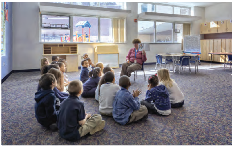
New Classroom on the southwest side of the school. Light shelves are utilized to increase the amount of daylight into the interior spaces.
